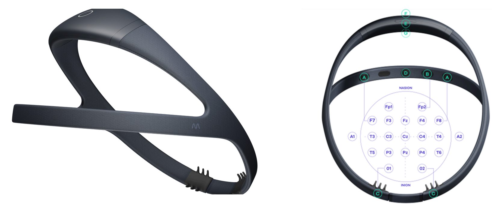
Waveband headband montage includes two frontal and two occipital contacts and is optimized for sleep comfort.
