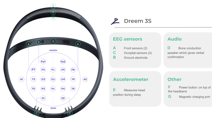
Figure 2: Dreem 3S headband and sensors
