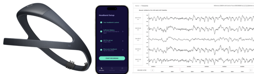
Figure 1: Dreem 3S headband, the Beacon Pal App, an EDF output of the device (left to right)
